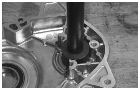
Refit the spring/toothed sector unit, hold the crankcase in a perfectly horizontal and stable position, place the spring/toothed sector unit keeping it perfectly perpendicular to the bearing already fitted on the crankcase; if necessary, slightly hit the unit shaft end with a mallet and protect the thread by screwing in a nut.
