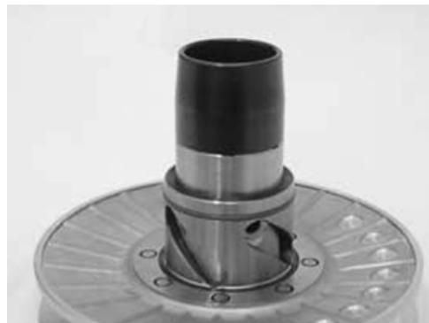
Using a curved-spout grease gun, lubricate the driven pulley assembly with approximately 6 g of grease. Apply the grease through one of the holes in the bushing until it comes out through the hole on the opposite side. This operation is necessary to avoid the presence of grease beyond the O-rings.
