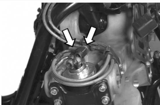
Remove the suspension tilt locking device pipes from the headstock.
