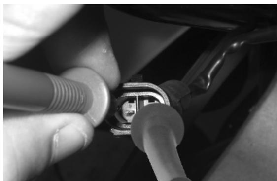
With interface wiring disconnected from the control unit, check the continuity between pin 34 and the brown cable of the tilt locking gripper sensor connector on the system side.
