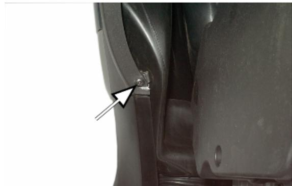
Remove the five screws on the right side and the five on the left side, indicated in the figure.
