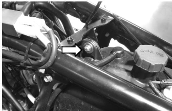
Remove the two lower bracket retainers indicated in the figure.
