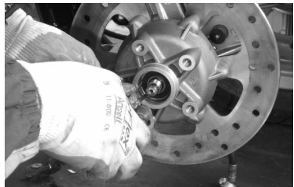
Loosen the 6 screws indicated in the figure and remove the brake disc from the wheel hub.
