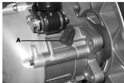
**UPON REPLACING HUB OIL, AVOID THE OIL COMING INTO CONTACT WITH THE REAR BRAKE DISC.**
