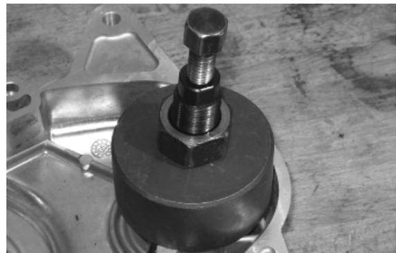
Hold the crankcase in a perfectly horizontal position, heat it with a heat gun at a temperature of about 120 °C, use the specific tool to fit the bearing of the spring/toothed sector unit. Hit slightly with a mallet if necessary.
