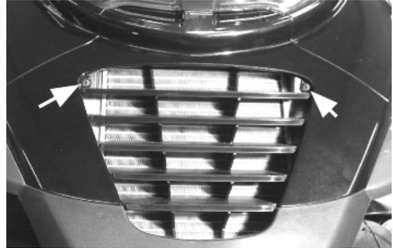
Remove the two lower retainers with the bushing
