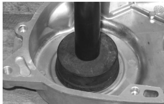
Hold the crankcase in a perfectly horizontal position, heat it with a specific heat gun at a temperature of about 120 °C, use the specific tool to fit the bearing of the electric motor. Hit slightly with a mallet if necessary.
