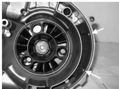
Align the drive with the reference on the crankcase cover.
