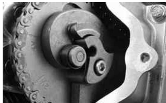
Assemble the limiting bell using the counterweight fixing screw as a reference.
