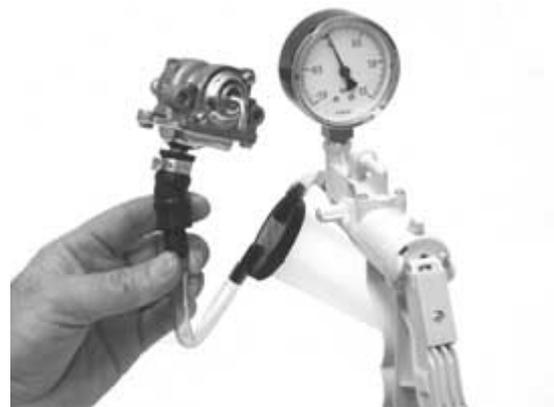
If anomalies are detected, replace the pump.
