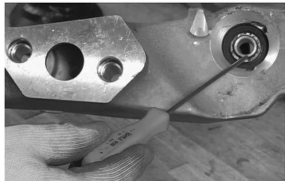
Check the inside tracks of the parallelogram bearings on the chassis.
