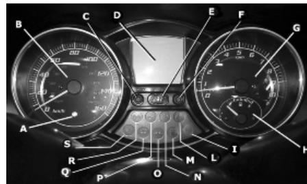
Q = Front suspension locking system failure warning light (if available)
