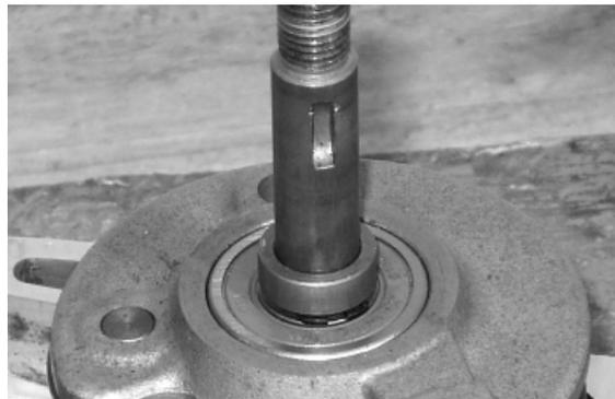
Lubricate the interference areas, match the crankcase halves with slight hits of a mallet to get them into contact.
