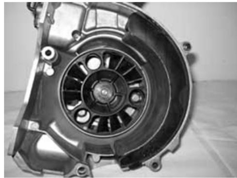
Undo the 3 fixing screws "A", remove the secondary air filter cover and then take out the filtering element "B".
