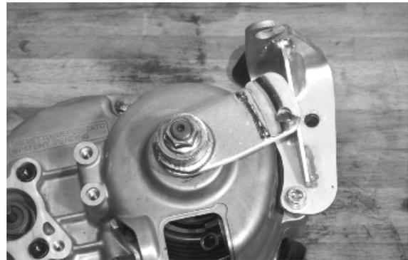
Refit the potentiometer (not forcing in the D-type connector ensures a sole position) with the connector directed to the opposite side of the hydraulic pump.
