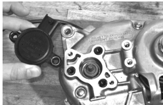
Remove the nut indicated in the figure, if necessary lock the lever with a vice making sure not to spoil the surface.
