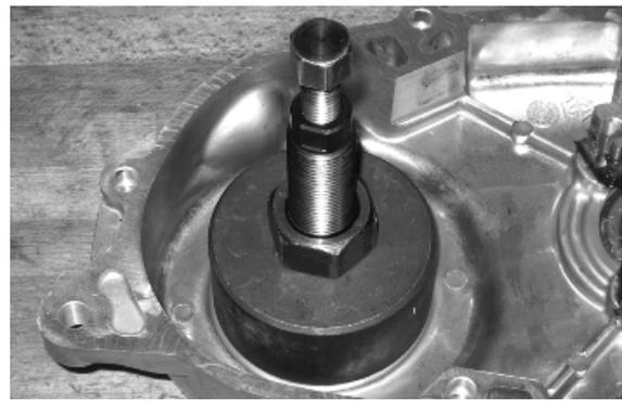
Extract the bearing of the electric motor with the specific tool.
