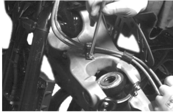
Remove the 4 screws fixing the tilt brake disc sector indicated in the photograph.
