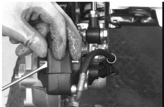
Remove the pad pin lock with a screwdriver, paying attention not to spoil the calliper surface treatment.
