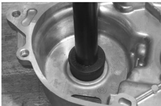
Hold the crankcase in a perfectly horizontal position, heat it with a heat gun at a temperature of about 120 °C, use the specific tool to fit the bearing of the electric motor. Hit slightly with a mallet if necessary.
