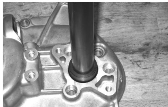
Hold the crankcase in a perfectly horizontal position, heat it with a heat gun at a temperature of about 120 °C, use the specific tool to fit the bearing of the flexible transmission lever control shaft. Hit slightly with a mallet if necessary.
