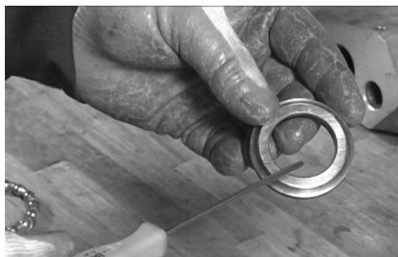
Check the ball bearings on the parallelogram arms. Replace them in case of signs of abnormal wear.
