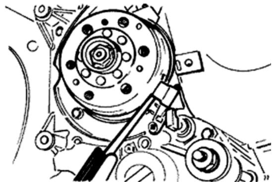
**Locking torques (N\*m)**Flywheel nut  $54 \div 60$
