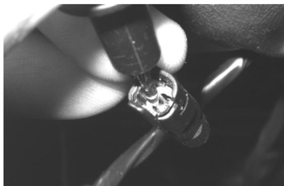
With interface wiring disconnected from the control unit and the connectors disconnected from wheel turning sensors, check that pin 23 - 17 and 24 - 17 are insulated from each other and from earth.
