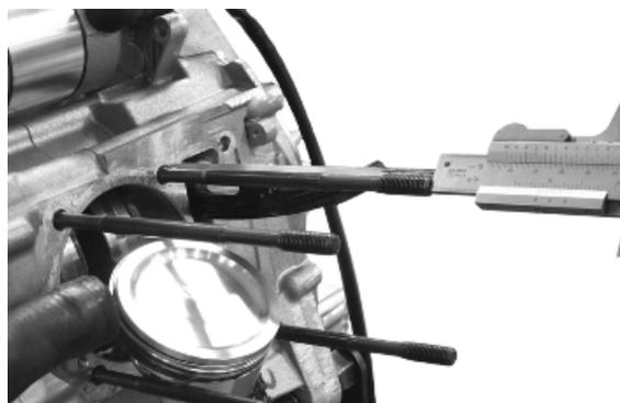
By working on two fitted cylinder head fixing nuts, nut and lock nut, as shown in the photograph, remove the stud bolt from its seat.
