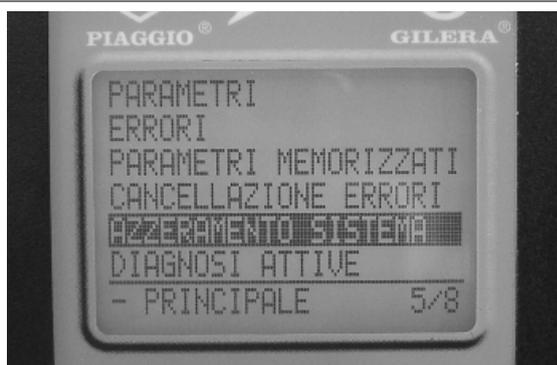
Select the POTENTIOMETER RESET option from the SYSTEM RESET menu and press OK.
