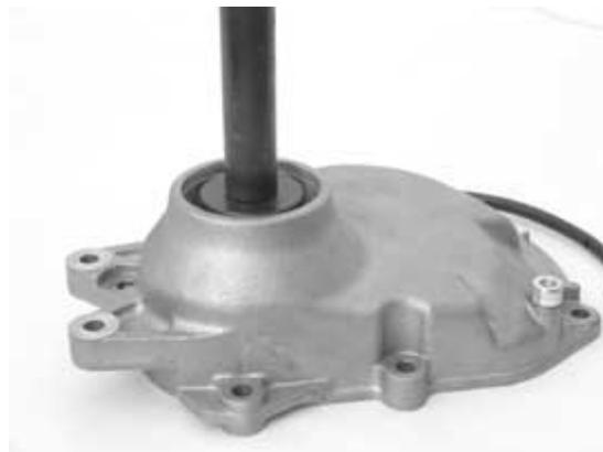
With the appropriate tools, remove the oil seal as shown in the figure.
