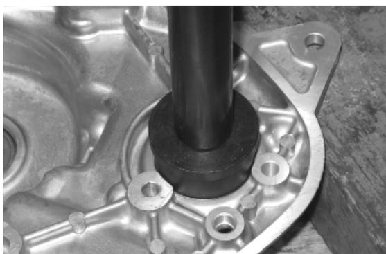
Remove the spring/toothed sector unit from its fitting, slightly hit with a mallet if necessary to release the unit.
