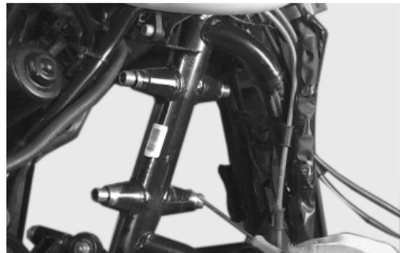
For refitting, follow the operations for removal but in reverse order, lubricating the locking pins on the parallelogram half-arms and observing the prescribed torques.
